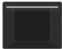
**Upper Heating Function:** The oven's thermostat and warning lights will switch on, and the upper heating element will start operating. The heat emanating from
