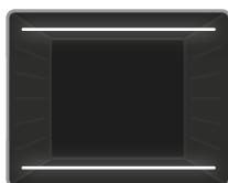
**Static Cooking Function:** The oven's thermostat and warning lights will switch on, and the lower and upper heating elements will start operating.
